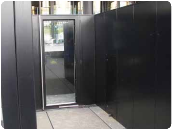
One-wing door: V2A/304 finish-painted in RAL 9005, internal hinges, extensively glazed, bar handle over the full door height, without header
