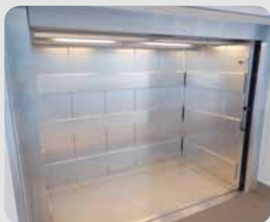
Floor with PVC knobbed surface, cabin walls made of stainless steel (V2A/304), impact protection from hardwood with V2A/304 cladding (three sides, three rows), ceiling with white light grill
