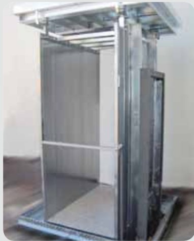
Basic structure and floor (checker plate) hot-dip galvanised, cabin walls hot-dip galvanised, no ceiling – only the roof frame, carriage zinc-powder primed
