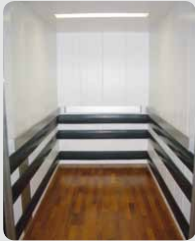
Floor as tray with customer-supplied lining, cabin walls and ceiling finish-painted in RAL 9010, handrail flat aluminium (all way around), impact protection black hard rubber (three sides, three rows)
