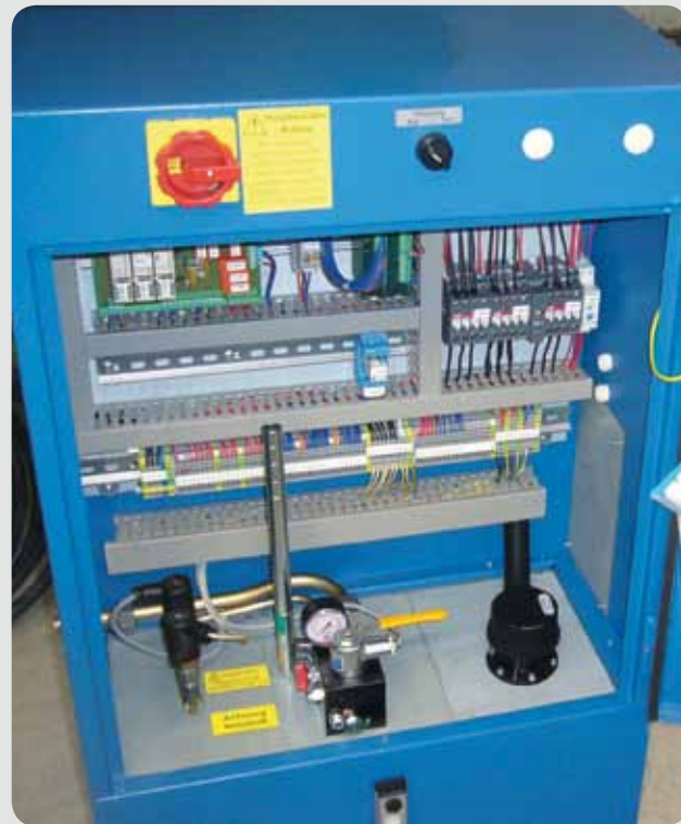
Open control cabinet. At the bottom, from left to right: pressure switches, control block and filling neck. In the middle, the control system; at top left the main switch
