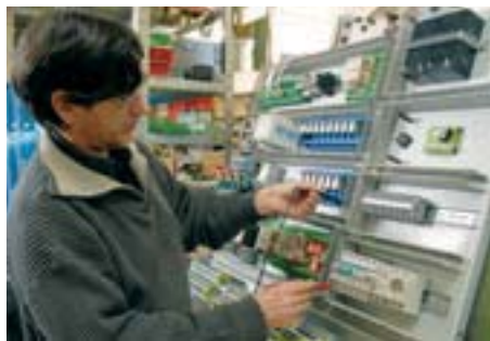
On completion, all controllers undergo a detailed and exhaustive test procedure (up to 21 pages long, depending on model).
