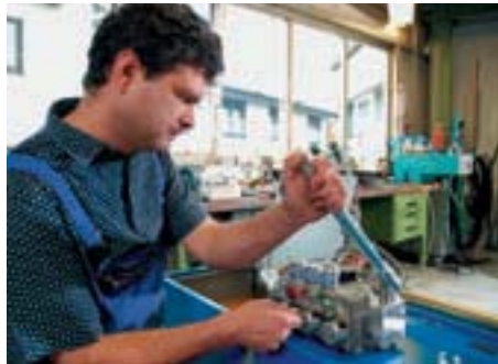
In the hydraulics department, Alexander Daum is responsible for assembling manifold blocks and fine-tuning the settings.
